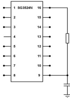
Figure 3: Soft start circuit for the PWM I
