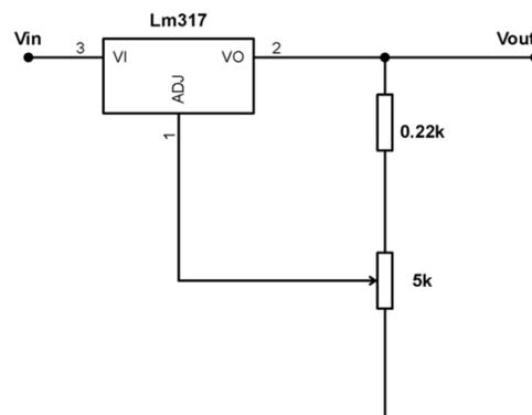
Figure 4: Voltage regulator circuit for USB port
