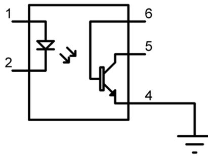
Figure 5: Opt-coupler Feedback control circuit
