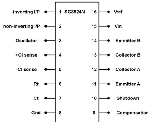
Figure 2: Diagram showing Pin configuration of SG3524 PWM IC
