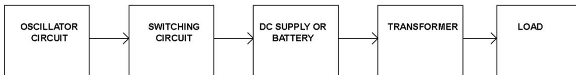
Figure 1: Block diagram showing basic working Principle of an Inverter
