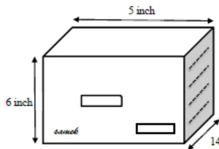
Figure 7: A diagram showing the constructed inverter casing
