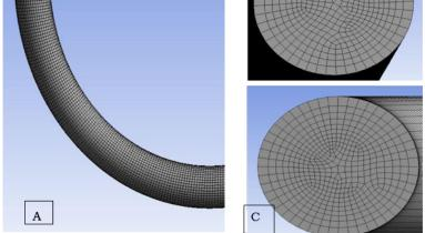
Figure 3: A picture of generated mesh; (a) bend section; (b) Inlet section (c) Outlet section
