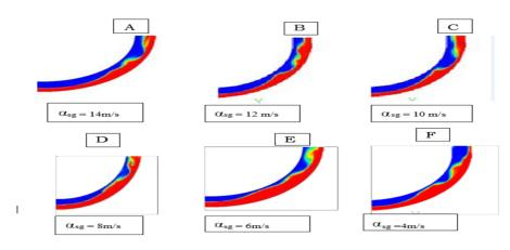
Figure 5: Contours showing the nature of flow along the bends
