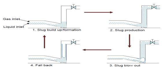
Figure 1: Severe slug Stages/cycle phenomenon adapted from Taitel (1986) and presented by Ogazi (2011)
