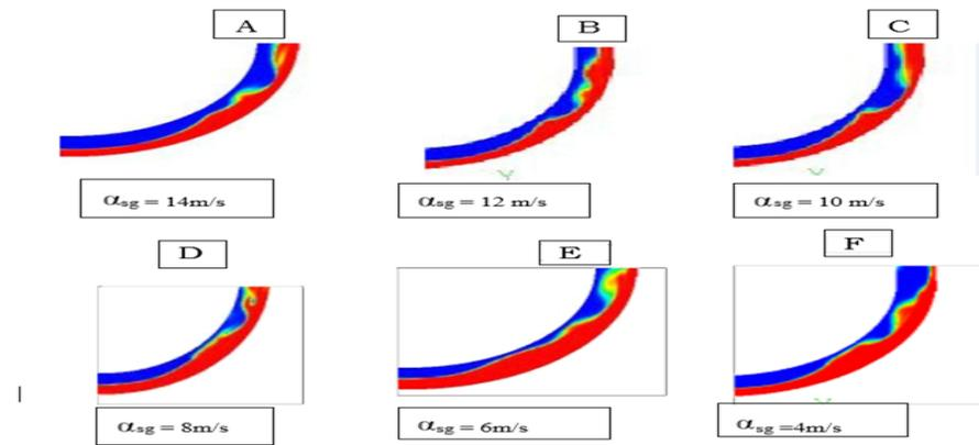
Figure 5: Contours showing the nature of flow along the bends
