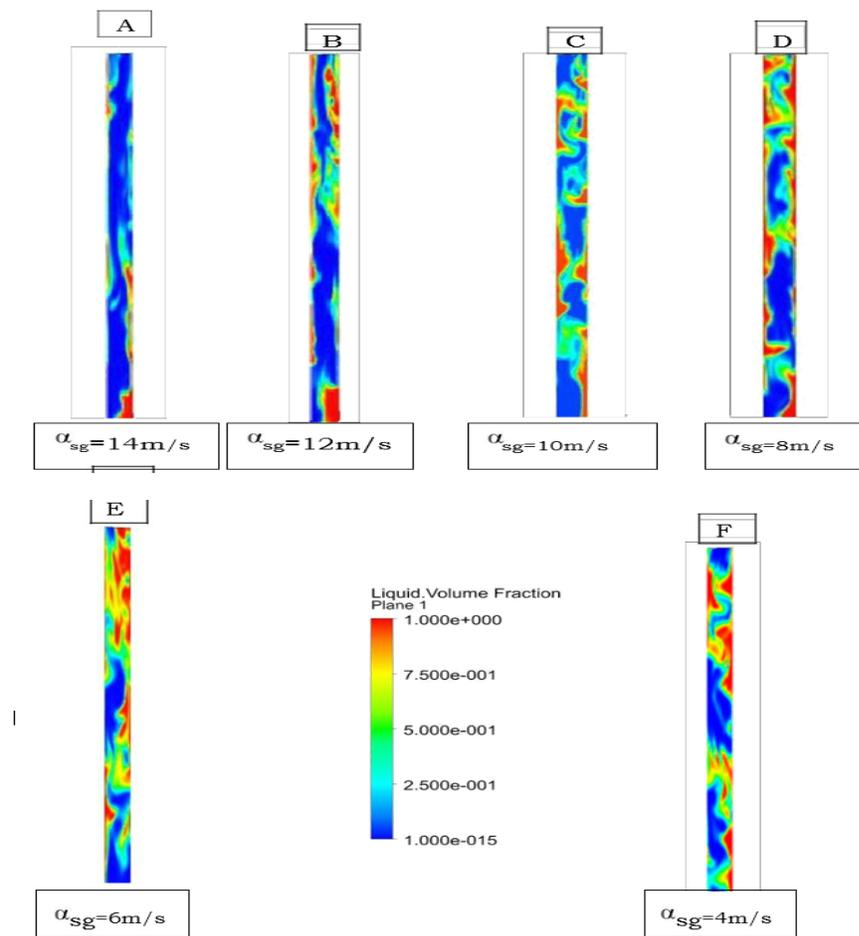
Figure 6: Contours showing liquid volume fraction in the vertical riser for all the tested superficial velocities
