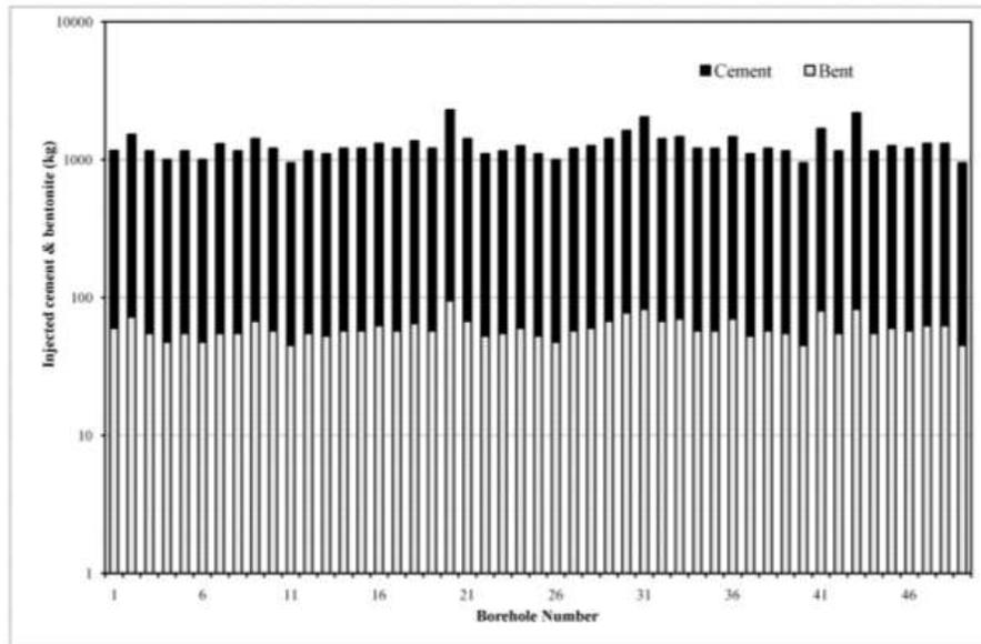
Figure 3: Sum of injected cement and bentonite at site M
