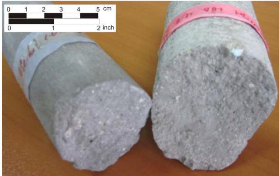
Figure 4: Some core samples of grouted soils
