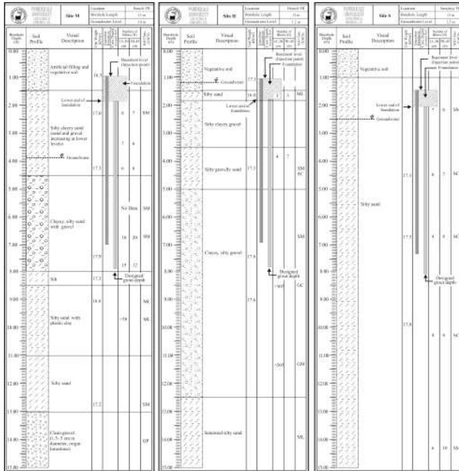
Figure 2: Borehole logs from the sites
