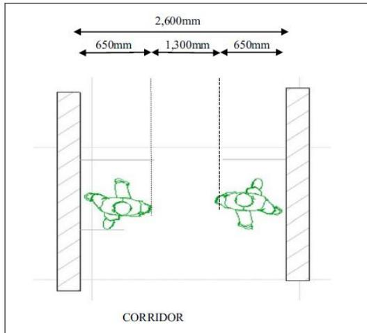
*Fig. 3: Suggested minimum Corridor width (Emmanuel et. al., 2020)*
