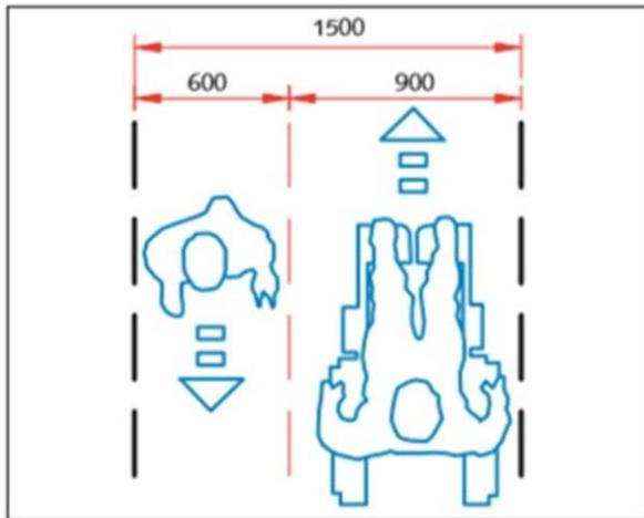
**Fig. 1:** Corridor width as recommended by UKDH (2013)
