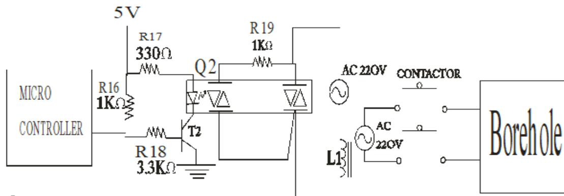
**Figure 7:Block Diagram Showing Borehole Control Sub-Circuit**
