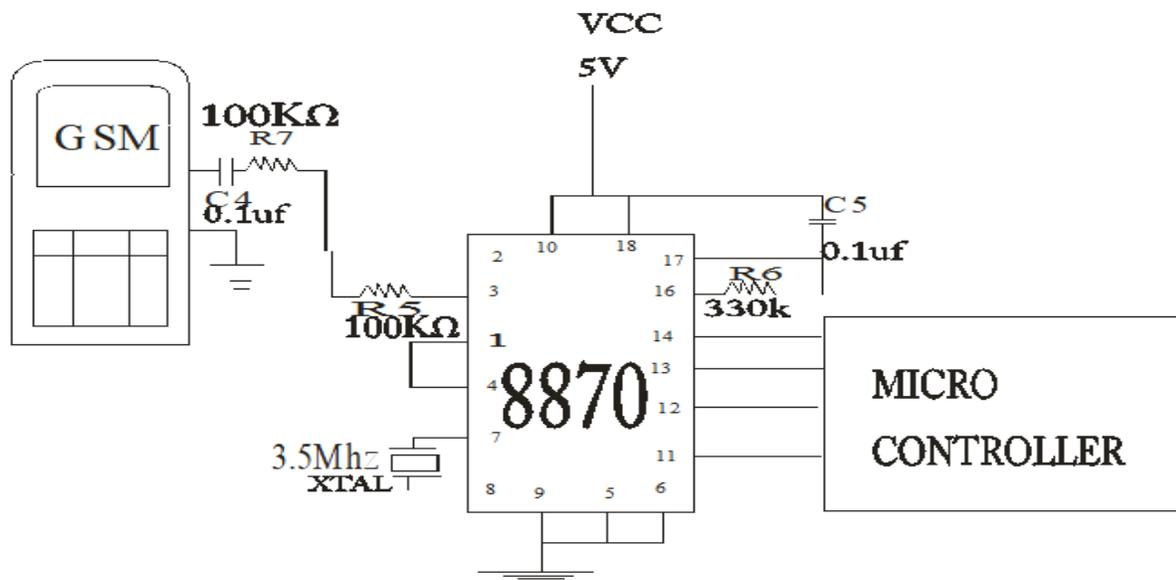
Figure 3: Block Diagram Showing Gsm Receiver Sub-Circuit
