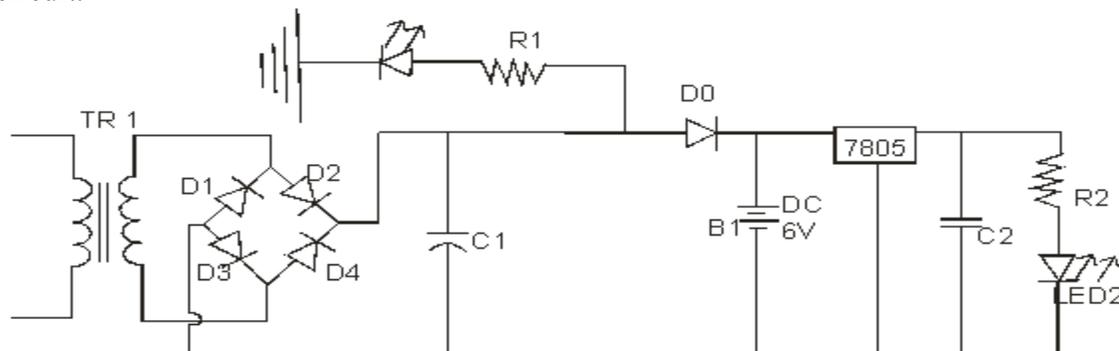
*Figure 1: Block Diagram Showing Power supply unit/ battery charger unit*
