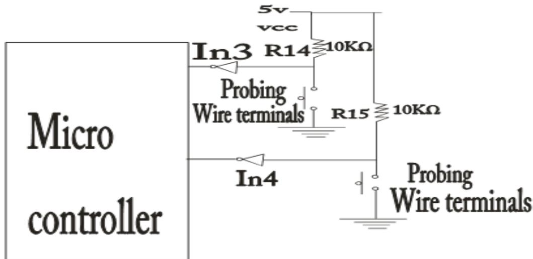
**Figure 6: Block Diagram Showing the Feedback Sub-Circuit**
