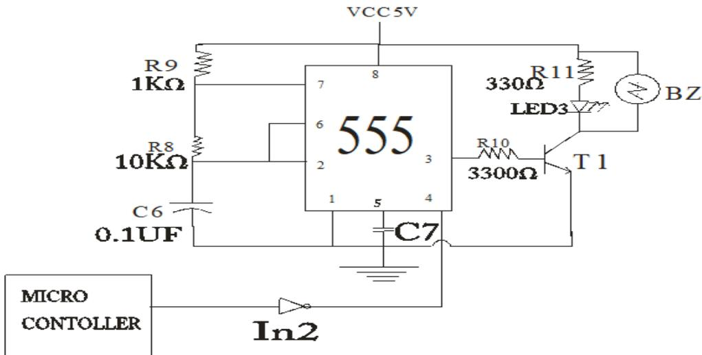
Figure 4: Block Diagram Showing Alarm sub-circuit
