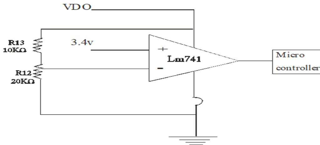
Figure 5: Block Diagram Showing Voltage Monitoring Sub-Circuit
