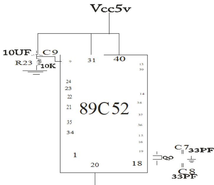
**Figure 9: Block Diagram showing Micro Controller Sub-Circuit**
