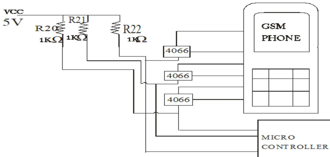
**Figure 8: Block Diagram showing Gsm Transmitter Sub-Circuit**
