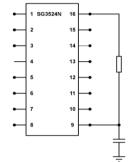
Figure 3: Soft start circuit for the PWM I
