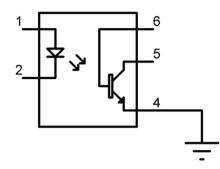
*Figure 5: Opt-coupler Feedback control circuit*
