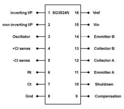
Figure 2: Diagram showing Pin configuration of SG3524 PWM IC
