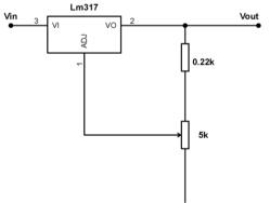
Figure 4: Voltage regulator circuit for USB port
